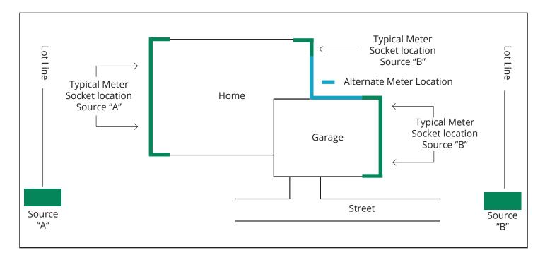
Meter Socket Requirements: All meter sockets must be a minimum of 200 amp with a lever bypass.
